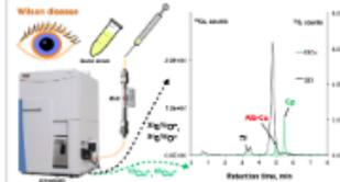
**ANCC Determination:** Serum proteins were separated by anion exchange chromatography and copper content of protein peaks determined by ICP-MS. Internal standardization is possible using natural sulfur and copper isotopes.
